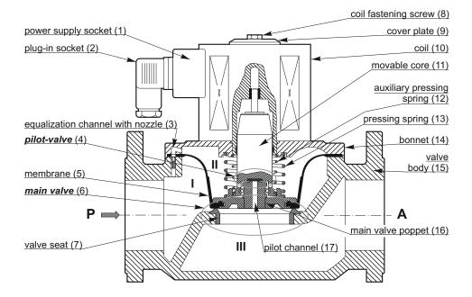
When describing the operation of the ZEF valve (with assisted lift), we distinguish two cases:
