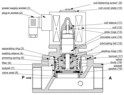
(\*) in valves ZEAb special cover (9a) fastening coil act as coil fastening screw (9) - see p.7.
